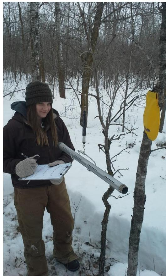
Establishing weight of snow sample to calculate water content
